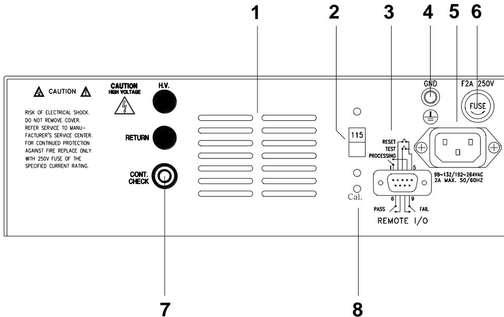
1. **THERMAL FAN:** To cool the instrument.
