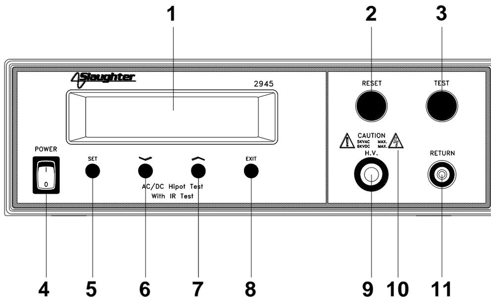
7. **UP ARROW (^):** Use this key to increment numeric values in the setup mode. This key also used to toggle ON/OFF functions. Also may be used to increase output voltage during a test in 10-volt increments.
