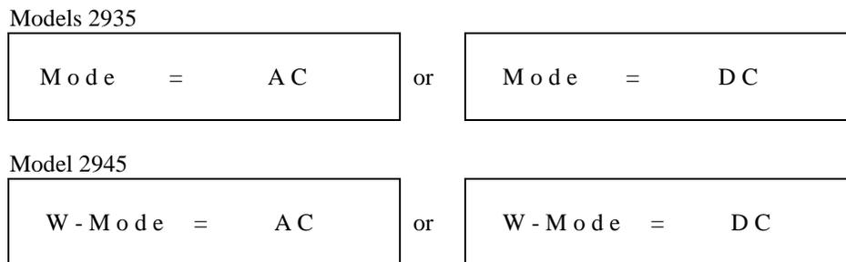
Press the Up or Down Arrow keys to toggle the output function; AC or DC, then press the EXIT key to exit to the test mode or toggle to another setting using the SET key.
