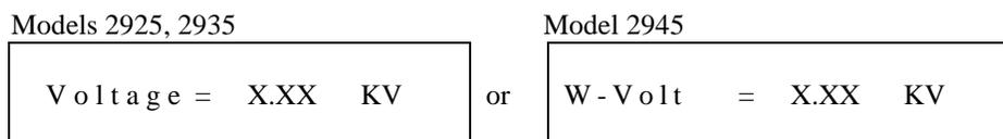
Please use the Up/Down Arrow keys to enter the desired test voltage, then press the EXIT key to exit to the test mode or toggle to another setting using the SET key. The maximum voltage which may be entered is 5000 volts AC or 6000 volts DC.
