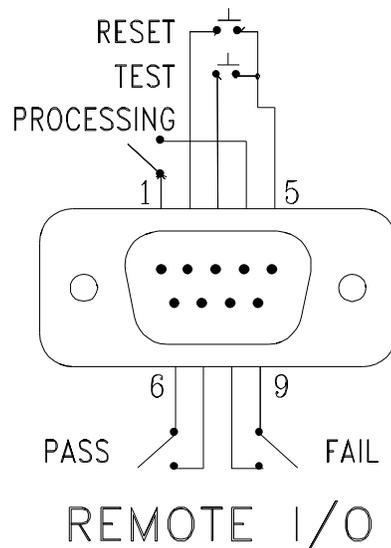
and PROCESSING conditions. These signals are provided by three normally open internal relays that switch on to indicate the current condition of the tester. These are normally open free contacts and will not provide any voltage or current. The ratings of the contacts are 1A / 250 VAC ( 0.5 ADC ). Below is a listing that indicates what conditions activate each pin. When a terminal becomes active, the relay closes thereby allowing the external voltage to operate an external device.
