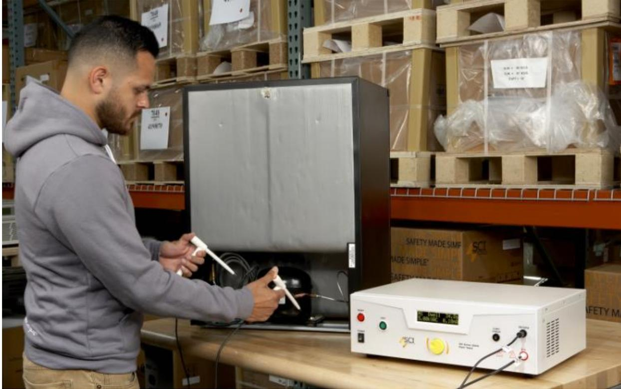
The 298 instrument's voltage regulation circuitry ensures that the output voltage will not dip under any line or load conditions. Additionally, the 298 meets the 200 mA short circuit current requirement called out in various product safety standards. These features, along with an intuitive user interface, make the SCI 298 a versatile yet simple hipot instrument.
